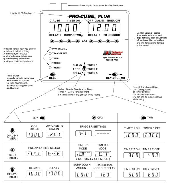
FACTORY DEFAULT SETTINGS FOR MODEL PCT3-P ARE SHOWN IN THIS TABLE (SEE "TIMER OUTPUT CONFIGURATION" SECTION FOR MODEL PCT1-P)
