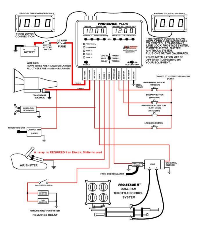
Wiring Diagram – Complete System for PCT3-P with 3 Timers
